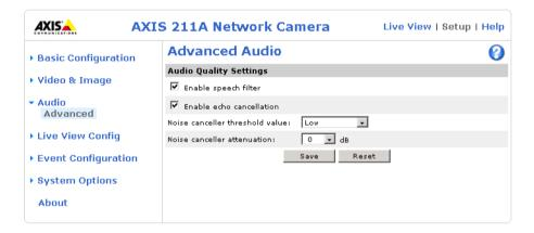
Enable speech filter improves the sound quality when the microphone is placed close to the person talking and can also help reduce background noise. The filter cuts the lowest and the highest frequencies. The bypass frequency range is approximately 250Hz to 3700Hz (measured at -10dB cut-off break points).
