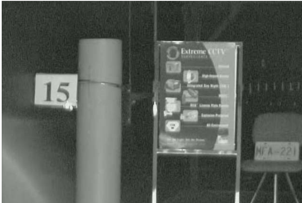
Trial 11: infrared off. Ambient visible lighting 1.04 lux. Bit rate = 5.27 mbps.
