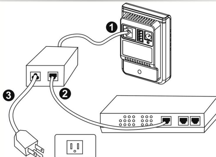
5. Use a standard Ethernet cable to connect the camera to a PoE Injector.
