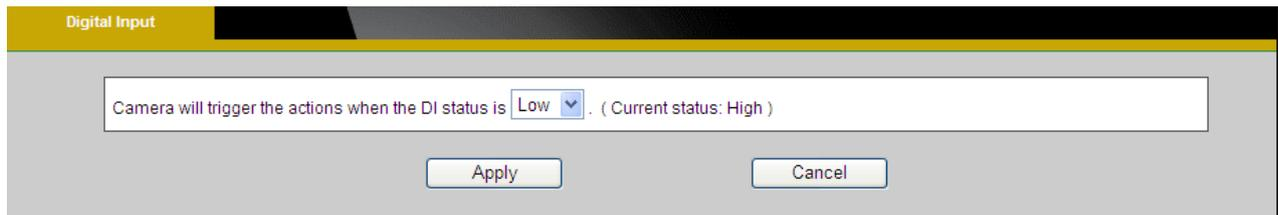
The DI socket allows the IP camera to receive input from an external device.
