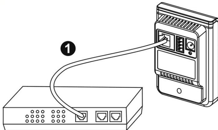
1. Use a single Ethernet cable to connect the camera to the PoE-enabled switch.
