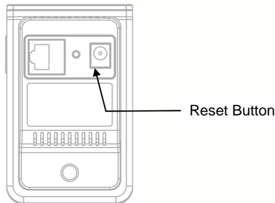
The Reset Button can be used to reboot the camera or restore it to factory default settings. If the camera experiences a problem, rebooting the camera may correct the problem. If the problem remains, please restore the camera to factory default settings and reinstall the software.
