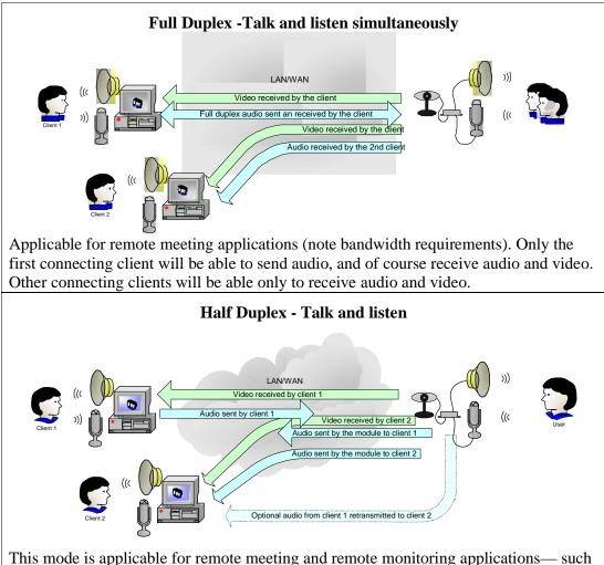
This mode is applicable for remote meeting and remote monitoring applications— such as entrance systems. In this mode, a special setting is available for re-distributing the audio stream from one client to another. This setting can prove particularly useful where single speaker control is desirable, i.e. within remote guidance scenarios.
