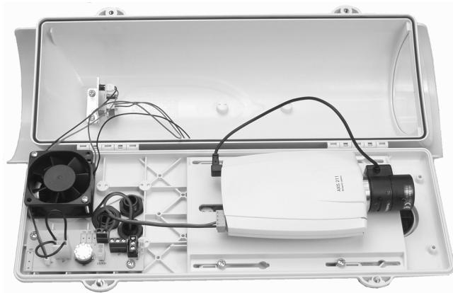
This document is an addendum to the **Camera Housing Operating Instructions** and describes how to connect power to a Axis network camera installed in the housing. Please read through both instructions before proceeding with the installation.
