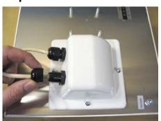
Place Sealing Gasket over screws.
