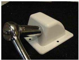
Tighten using a <sup>3</sup>/<sub>4</sub>" wrench or socket. Tighten until the Cable Lock touches the Boot as shown in Step 3.
