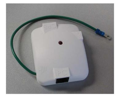
Connect the power adapter to the power socket on the Power over Ethernet Adaptor (POE), and plug the other end of the power into an electrical outlet. Plug the RJ-45 Cable from the unit into the POE. The Station Adaptor will be powered on and the power indicator on the top panel will turn on.
