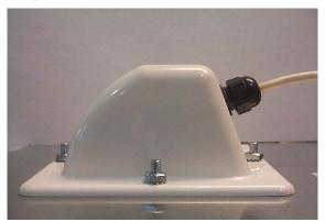
Place the Ethernet boot over the 4 Screw Posts. Apply 4 Kept nuts to the screw posts and tighten until the gasket makes full contact with the Ethernet boot. The gasket should be at least 50% compressed.
