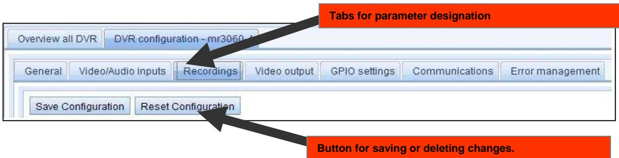
The two main tabs from the top row cannot be closed. The configuration of the system is built around a logical sequence (from left to right):
