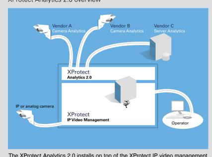
The XProtect Analytics 2.0 installs on top of the XProtect IP video management software and handles both analytics at the edge (in the camera) and server-based. The operator accesses all video analytics from one single user interface.
