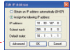
Easy assignment or change of IP address
