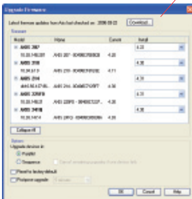
Single or multiple Axis video products of different models can easily be firmware upgraded sequentially or in parallel
