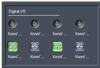
The round alarm icons (in the top row of the example) indicate the status of an alarm input for information purposes. If an alarm exists, the corresponding icon lights up. The configuration of the remote station determines whether alarms are displayed or not.
