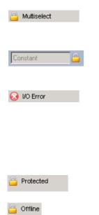
If several devices are selected, some settings cannot be made. The input fields are marked with a padlock.
