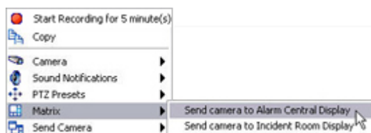
Example: Sending a camera's images to a Matrix recipient through the shortcut menu
