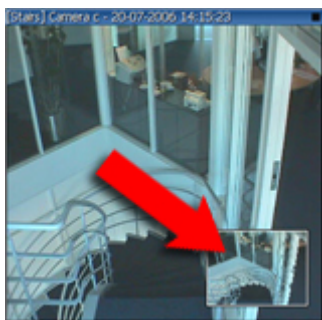
Overview frame inside image
