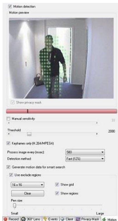
Camera properties: Motion tab with red deflection on the motion indication bar
