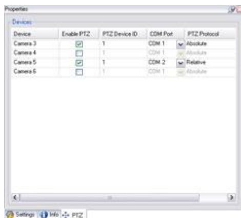
PTZ tab, with PTZ enabled for two channels on a video encoder
