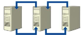
*Server clustering* -- A common server clustering method is to have two servers work with the same storage device, such as a RAID system. When one server fails, the other identically configured server takes over. These servers can even share the same IP address, which makes the so-called "fail-over" completely transparent for users.
