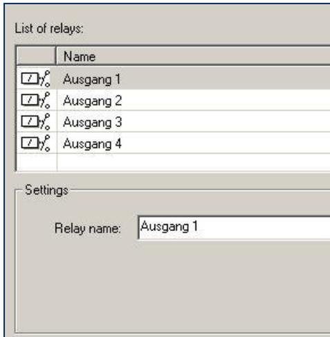
Relays which are to be switched by the recorder can be connected to its digital outputs.
