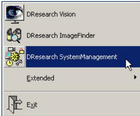
The CMS consists of the modules Vision, ImageFinder and SystemManagement. Only the system management module is relevant for the configuration of the recorder. There is a detailed description of the CMS software in the software manual.
