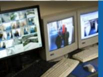
Two AXIS 241Q Video Servers with four analogue cameras on each are deployed to take images from existing analogue cameras and relay them into the network. A total of 18 AXIS 211 Power-over-Ethernet Network Cameras, and one AXIS 2130 PTZ Network Camera were deployed across the entire campus. A total of 27 cameras feed into the Milestone XProtect Enterprise Version 5.0 system for handling, storage and management of camera output.
