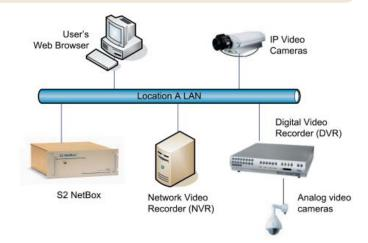
All components are connected to the network. Both IP and analog cameras are supported.  $\,$
